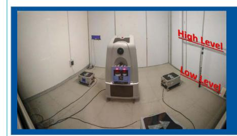
**Pictured:** Example of high and low level placements for test samples
